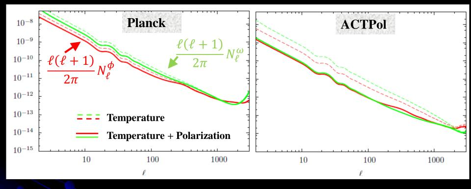
Note: For ACTPol, the noise improvement by including polarization is significant compared to that of Planck
